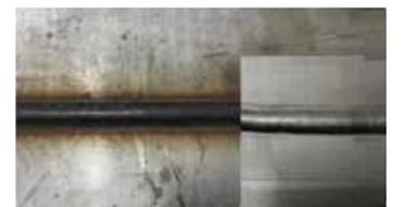
Pretreatment of welding surface and spraying surface
